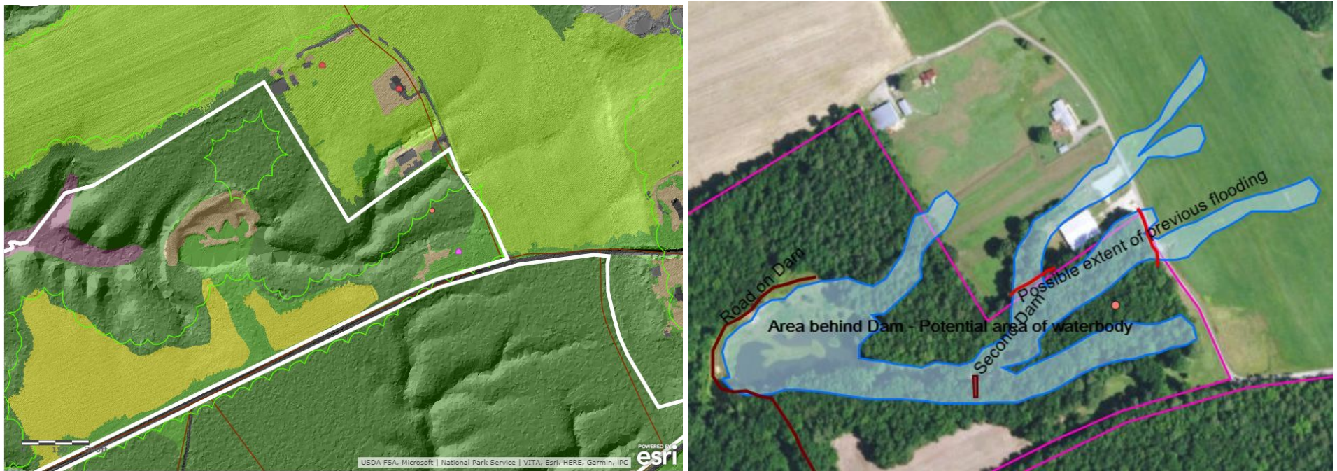
Figure 13: Left image: WERO as depicted in ArcGIS Online NPS layers and tools, including boundary survey (white line), LIDAR hillshade, and Virginia Land Cover data. The elevation difference between the dam and the downstream channel is evident in this image. The filled red circle indicates a spring. The headwaters appear to be springfed and those of the portion of Leigh Creek feeding the dam pond begin on the neighbors' properties in the northeast / top right corner of the image. Right image: Freehand drawn impoundment area behind the downstream dam (in blue), road and downstream dam (in brown), approximate location of second dam (brown rectangle), and reported extent of previous flooding. Note location of red circle indicating spring on the top of the hill between tributaries. Spring locations requires verification.
