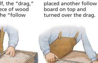
board," placing the He then removed the wooden pattern infirst follow board. side. He then sifted blew away loose sand from the edges of the fine sand over the pattern and packed pattern with a belthe rest of the drag lows 3, and "dressed" with coarse, damp the edge with a sand 1. After scraping moulder's spoon. He attached the "cope." away excess sand with the "strike" 2, he the flask's top half, to the drag and again added fine and coarse sands. Before packing
