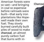
tense heat. The great demand for charcoal meant that early furnaces were sited on woodlands. One other ingredient was needed: air. It was directed into the hearth under pressure by the water powered blast machinery, raising the fire in the furnace to smelting temperature.
