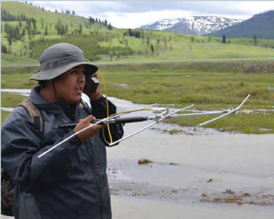
Citizen scientist using radio telemetry to locate collared bison (Photo: Ecology Project International)
