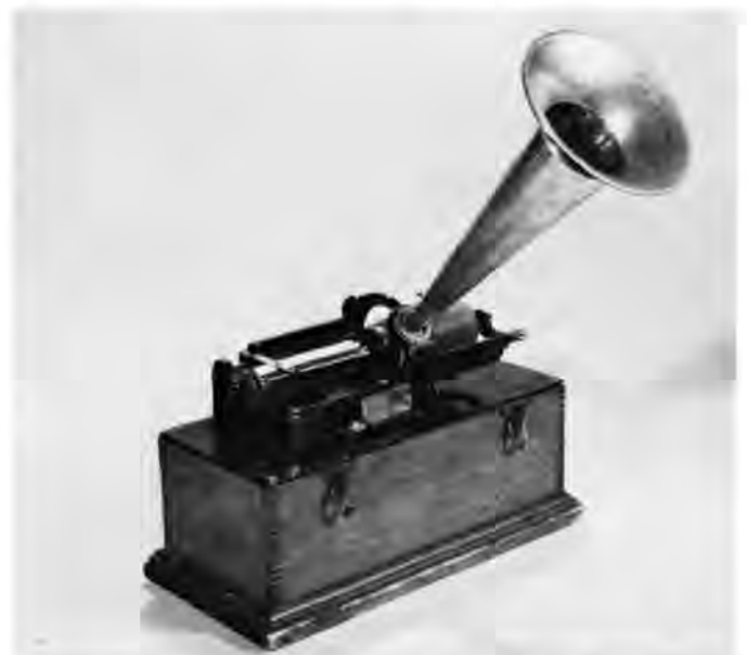
A cylinder phonograph machine. A person spoke or sang directly into the recording horn. The needle attached to the membrane at the bottom of the horn incised grooves onto the horizontally positioned spinning wax cylinder. American Folklife Center photo.
