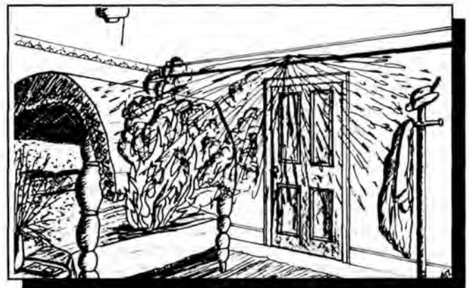
Guest room protection using sidewall residential sprinkler supplied by plastic pipe concealed in a boxed-in cornice. Maramede Inn, Middletown, MD.
