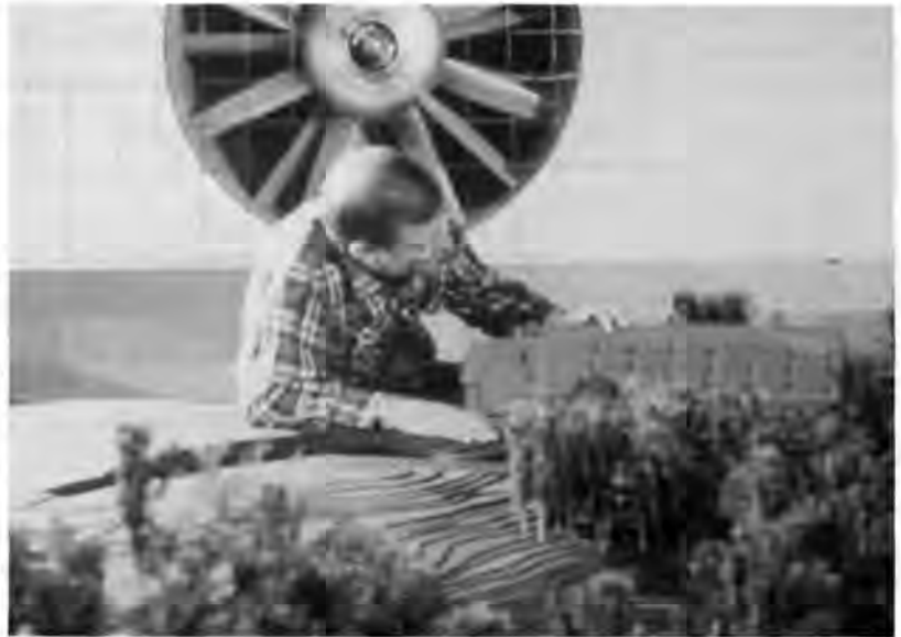
Figure 3. Wind tunnel testing can be useful in predicting the behavior of snow around a building.
