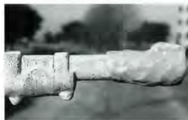
3. Molds were taken of the semi-cylinder below the front gunsight using ESPE Permagum Elastomeric Vinyl Polysiloxane Impression Material, developed for taking dental impressions. This is a two-part putty that consists of a base paste and a catalyst that, when kneaded together, form a putty that replicates complex surface textures. The putty sets up into a rubbery state in two to five minutes and remains pliable enough for easy removal. Because the material was formulated to work best at body temperature, it does not set up well below 60°F. Photos by D. Montagna.
