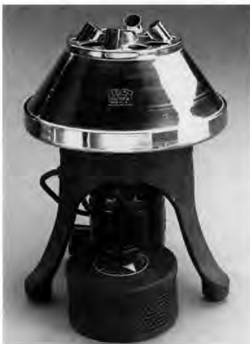
This Serval Angle Centrifuge, now part of the Stetten Museum Collection, was a handy desk top model used for small samples. Photo courtesy Stetten Museum.
