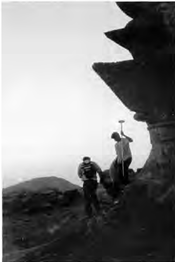
Establishing real world coordinates for points visible in all aerial imagery with a global positioning system (GPS). Photo by the author.
