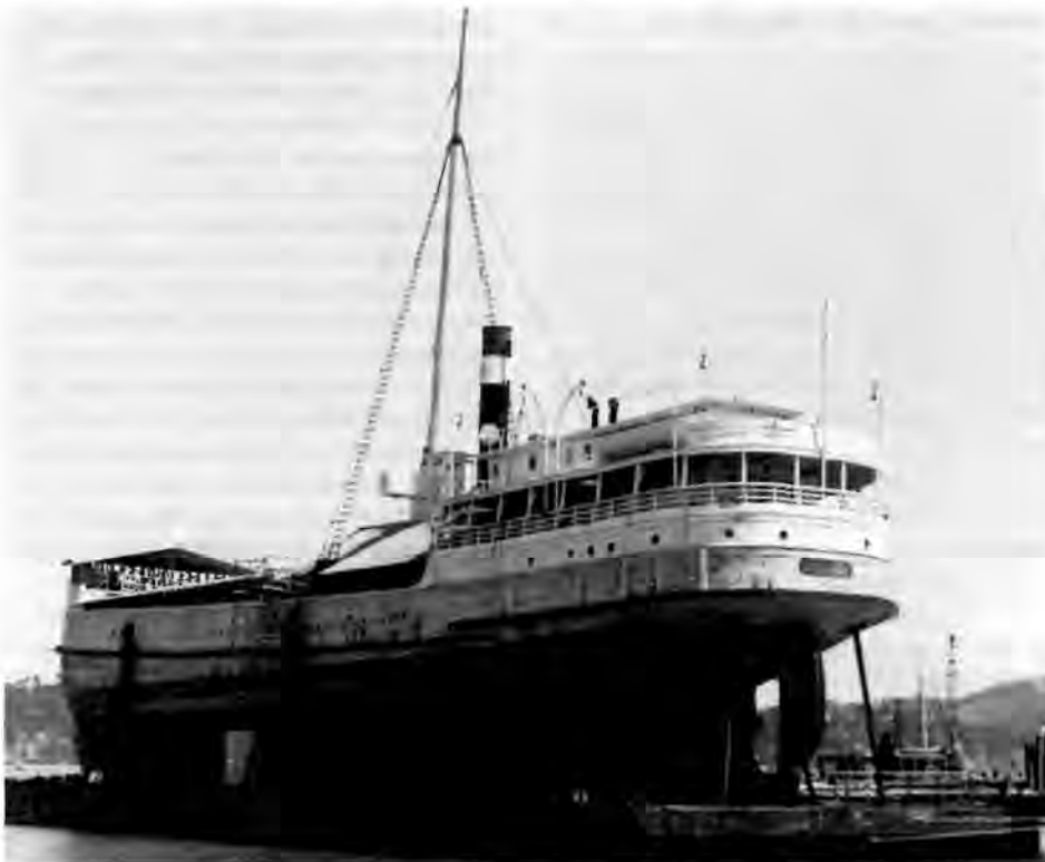
Wapama on her preservation barge with a protective roof over her decks, 1986. Photo courtesy of National Park Service/Richard Frear
