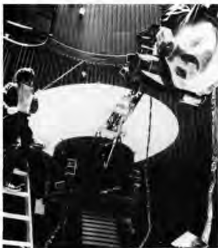
25-foot Space Simulator at the NASA Jet Propulsion Laboratory, Pasadena, CA, showing test of Voyager spacecraft, 1977. Photo by NASA Jet Propulsion Laboratory.
