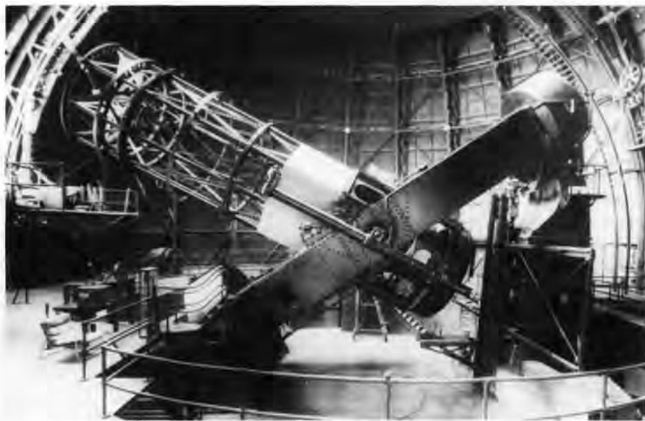
100-inch Hooker telescope of the Mount Wilson Observatory, Pasadena, CA, an international historical mechanical engineering landmark. Dominated discoveries in astronomy from 1918 until the dedication of the Palomar 200-inch Reflector in 1948. Contains many unique engineering features later incorporated into modern telescopes. Photo by Mount Wilson Observatory.
