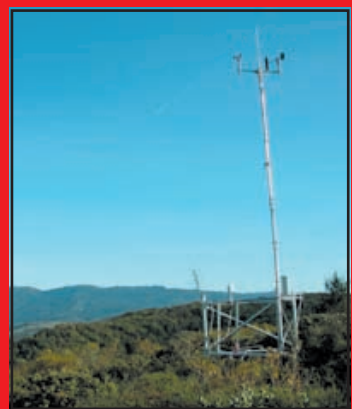
This new Remote Automated Weather Station (RAWS) will be used for fire weather monitoring by Marin County Fire Department and was recently provided through the National Fire Plan. There are two other RAWS stations in the county. The weather data from these stations can be viewed at www.met.utah.edu/mesowest .
