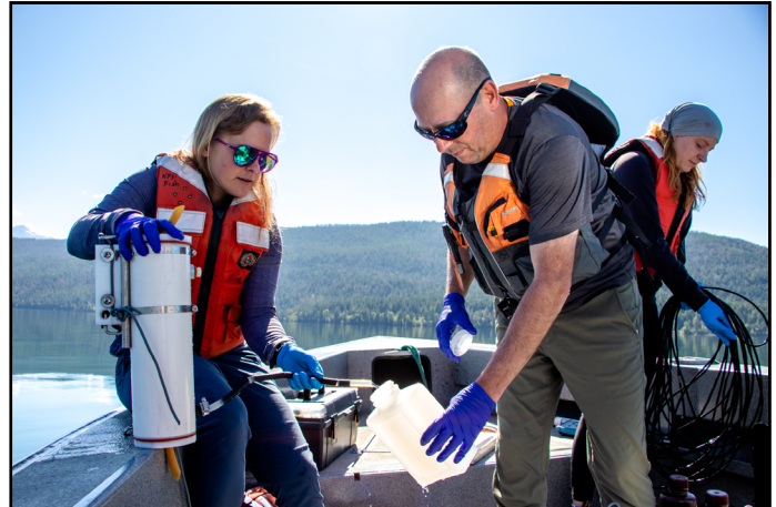
Researchers use a specialized bottle to collect water samples in Lake McDonald. Van Dorn Bottles (on the left in the photo) allow you to acquire samples from specific depths. NPS Photo/Kristin Vinduska
