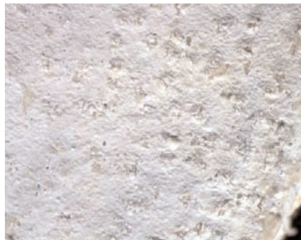
Fig. 8. Photographs taken with Leica MZ 8 stereomicroscope showing crystallization on the surface of limewash samples that included salt. The top photograph is of a handmade brick sample; the middle is a modern brick sample; and the final photograph is of a weathered wood sample. After drying, the crystallization became visually evident and was examined further under stereomicroscope.
