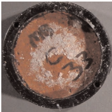
Fig. 9. Unexposed back of modern brick samples after artificial weathering. White residue was identified by Keymaster TRACer III Portable XRF as chlorine. The residue is evidence of salt migration through brick samples from the limewash in response to artificial weathering.
