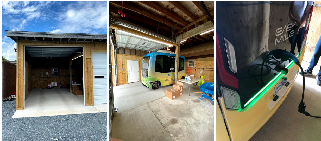
Figure 6: Shuttle Storage Garage Exterior (left), Interior (center), and Charging Equipment (right) Source: U.S. DOT Volpe Center
