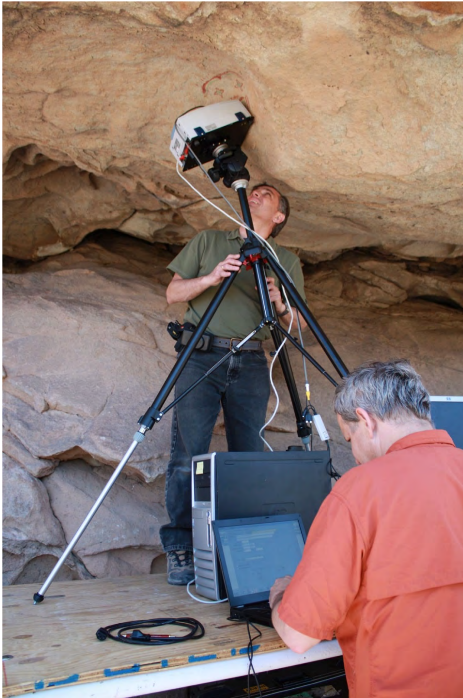
Photo 29. A team of professional conservators, scientists, and technicians using non-invasive techniques to identify the pigments and binders used to create one of the pictographs at Hueco Tanks. Analyses included portable X-Ray Fluorescence Radiography (pXRF), Raman Spectroscopy (Raman), and Fourier Transform Infrared Spectroscopy (FTIR). This was the first combined use of these techniques to analyze Native American pictographs.
